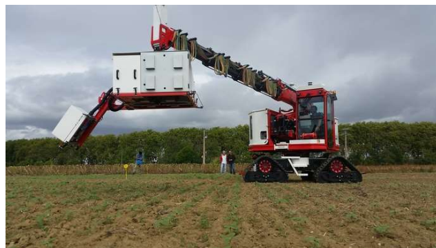
Figure 1. The phenomobile with caterpillars showing the 12m long boom supporting the measurement head.
